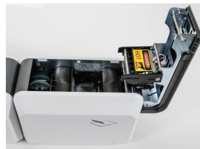
Figure 23 Installing the film cartridge
