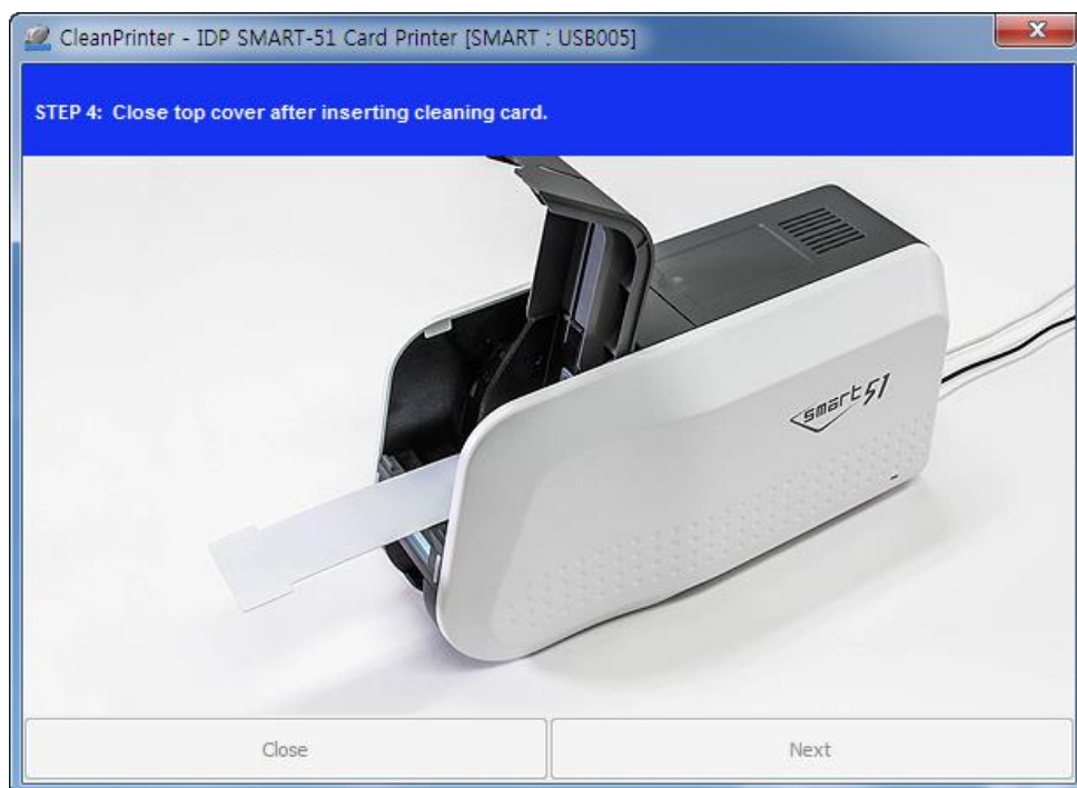
Figure 108 Printer cleaning Step 4
